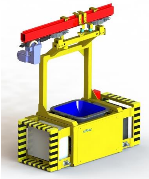
distribution car with monorail tracks with curves and switches possible
